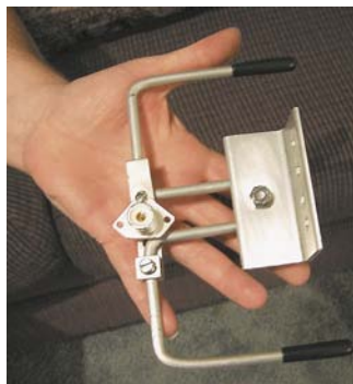
Figure 1—The 70-cm SQ loop antenna is less than 4½ inches across.
