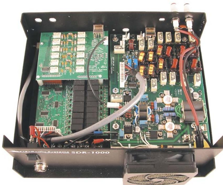
Figure 1—A look inside the SDR-1000 transceiver.
